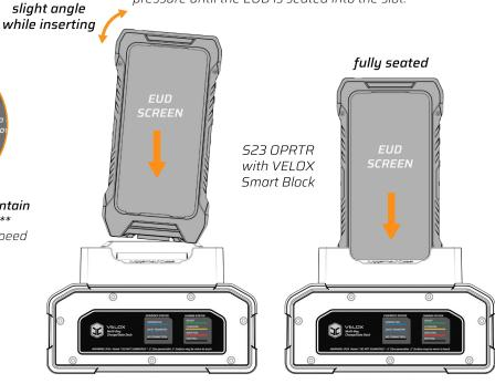
To remove, press down slightly, rock to the left or right until one side releases and then up and out.
