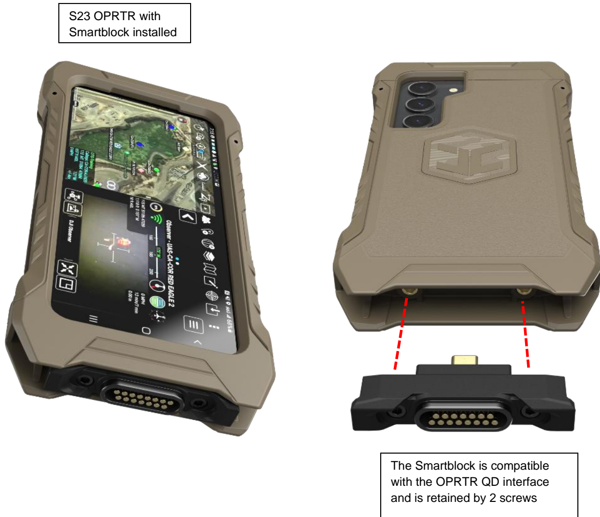
Fig. 4. OPRTR case with Smartblock shown
